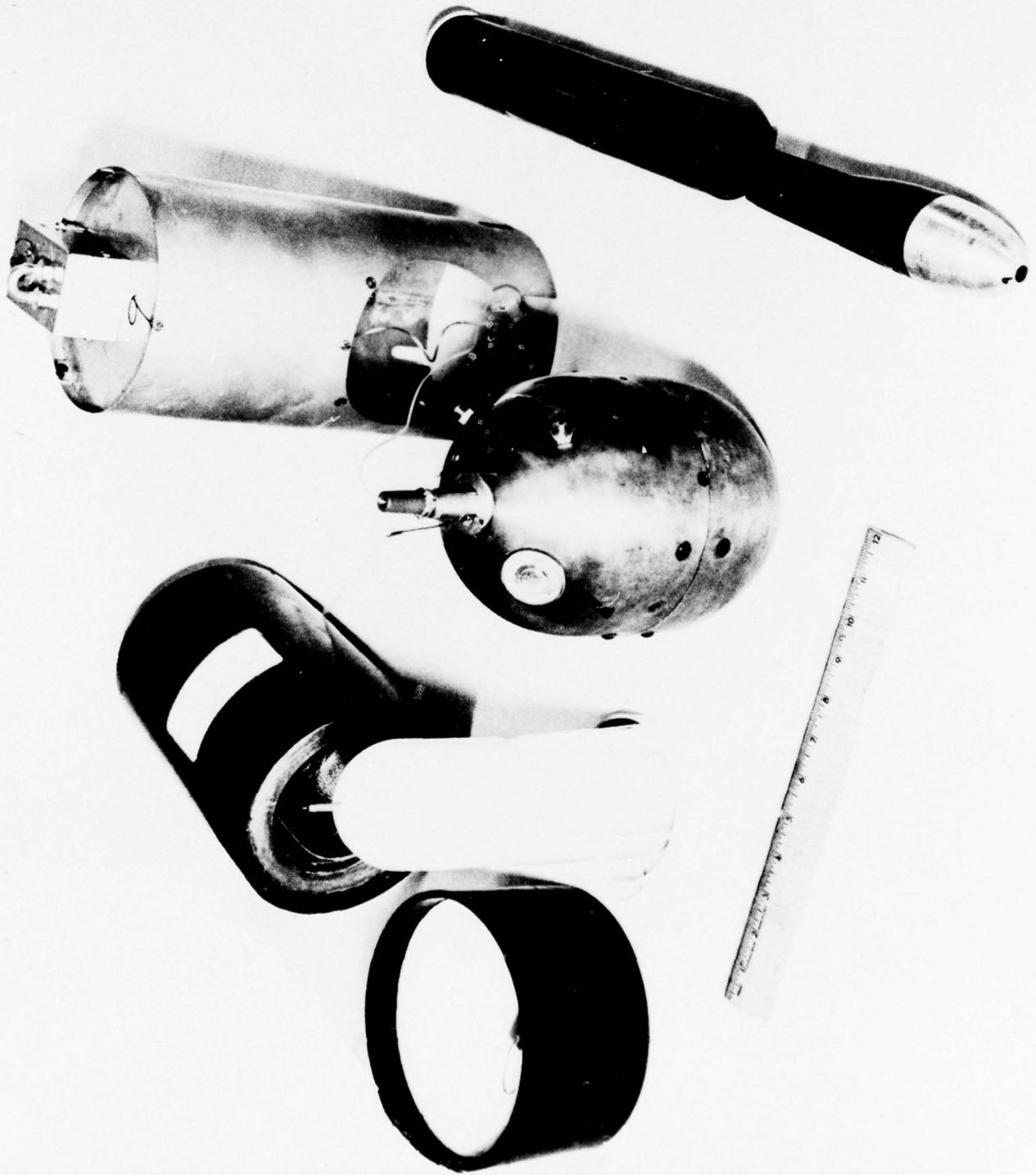
FIGURE 1 - EXPENDABLE BT UNITS, LEFT TO RIGHT - GENERAL MOTORS, BASIC DEVICES, FRANCIS ASSOCIATES
